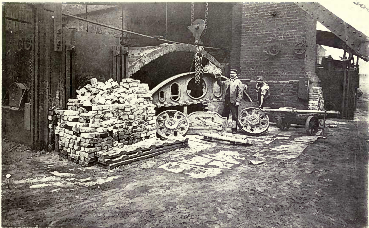
ANNEALING FURNACE AT EAST GUN WORKS BEING CHARGED.
