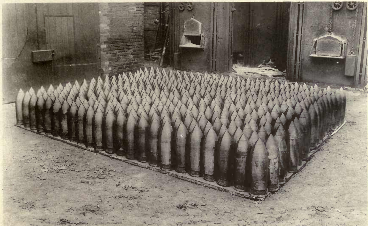
400 7.5in. CAPPED ARMOUR PIERCING SHELL, ACCEPTED AFTER FIRING TRIAL. READY FOR BANDING AND CAPPING.
